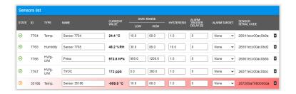
For the (2) Sensor disconnected scenario, you can also define an alert, -999.9 degrees Celsius means sensor not found and the device can alert you of this situation.
