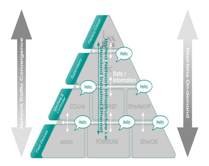
By implementing the autonomous pyramid of the Purdue model, manufacturers can realize their vision of smarkt manufacturing
