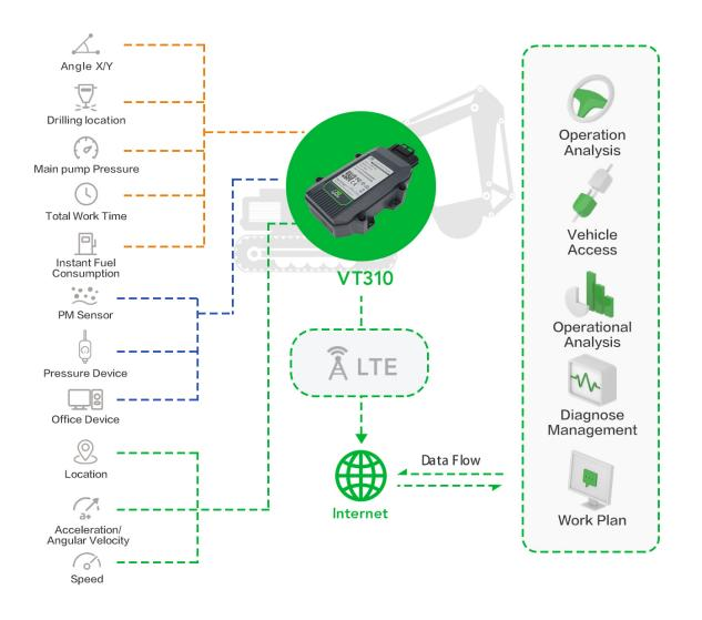
Featuring extensive I/O, standard protocols for communications and vehicle diagnostics, the VT310 can be connected to multiple peripherals on board
